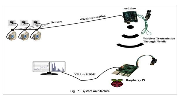
The test bed comprises of three computing devices. Initially, the real-time electric current values of the appliances are to be gathered. This is done with the help of CT (current transformer) sensors, one each clamped on every test device. The sensors are each of 5A capacity to withstand all the variations in the devices and give the electric current values in analogue form. This data is further passed on to the Arduino board through a wired connection.
