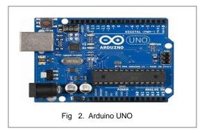
can be downloaded free of cost. The ATmega328 chip, initially, comes pre-programmed with the boot loader, due to which we can upload new code without any external hardware programmer. Hence, the biggest advantage of using this board can be that it saves us from a heavy task of circuitry building and tons of lines of coding by giving a pre-wired circuit and free code libraries.
